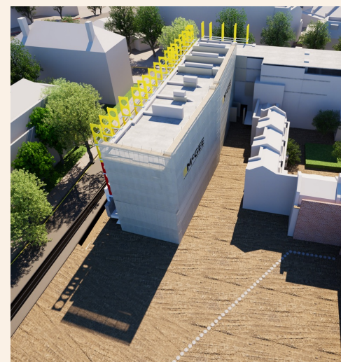
The façade retention system will be installed on the northern and western facades.
